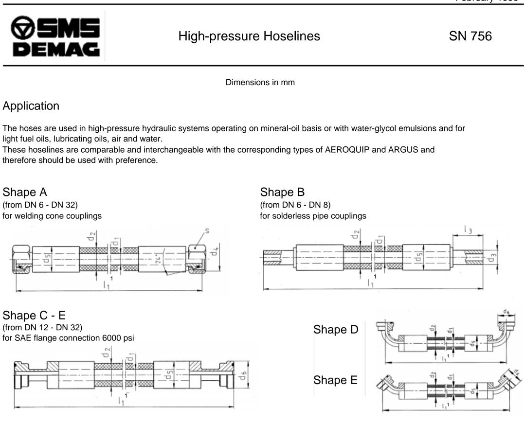
Designation of a complete high-pressure hoseline (4SH), shape A, nominal width of DN 25 and length 1000 mm:
